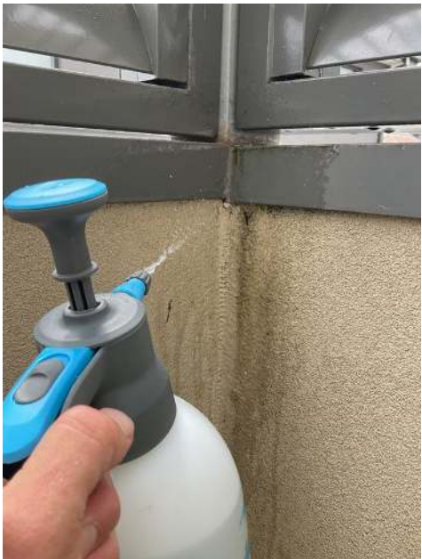
Hot water spray test
