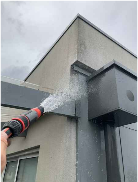
Hose test to render cracks and timber post to metal flashing connection
