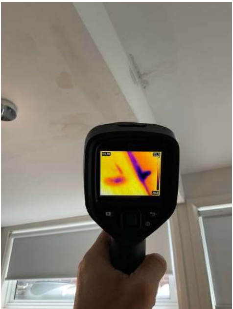
Hot water spray test over kitchen
