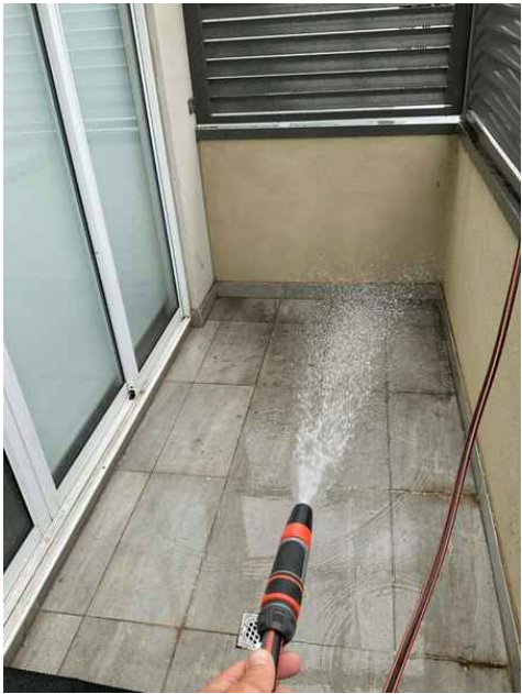
Hose test carried out to check ponding water and leak to garage ceiling
