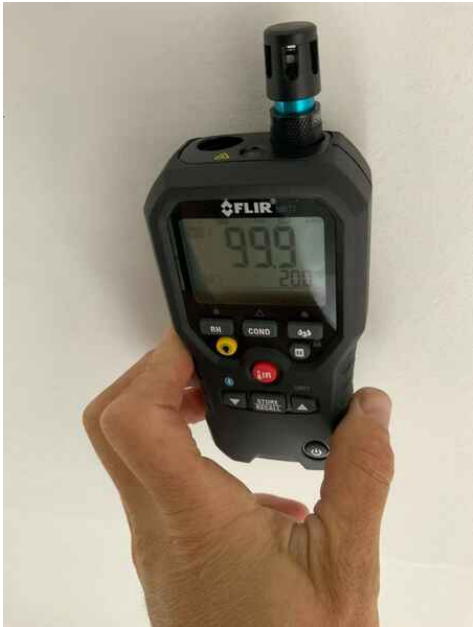
High Moisture Reading to Garage Ceiling at Leak No.2
